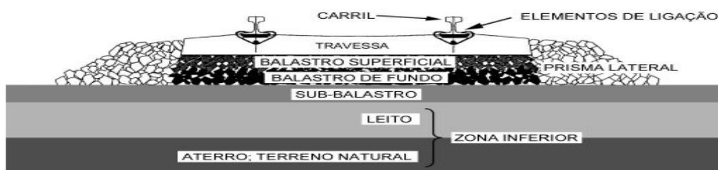
Figure 1. : Schematic cross section of ballasted track
